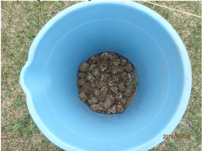
**Photograph-4:** View of a composite sample before being placed the laboratory supplied jars.
