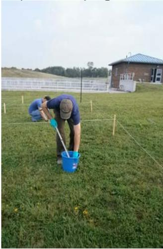
**Photograph-3:** View of GENIVAR field staff collecting the composite sample from the upwind sampling location.
