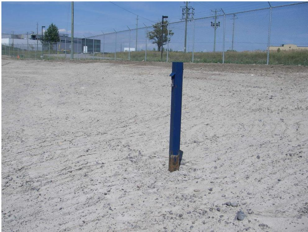
**FIGURE A-6:** Photo of Monitor MW4 following height adjustment.
