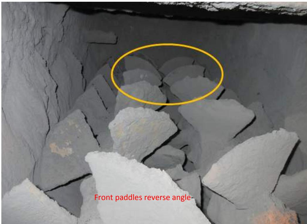
Photo 42 - Double Shaft Mixers – Some Paddles out of Proper Orientation
